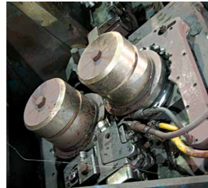
Heavy duty roll housing for thermomechanical rolling capability
