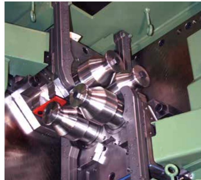
Close-centered sizing stands with new cooling headers
